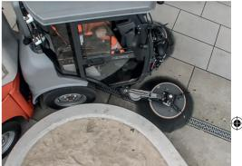
Gets in almost every corner: The steering system with articulated joint ensures excellent manoeuvrability – even when sweeping in reverse gear.
